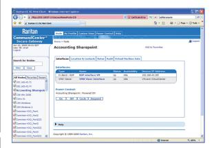
Stay connected to virtual servers even when they are moved from one virtual host to another. Issue on, off, cycle or suspend virtual power commands using the control buttons.
