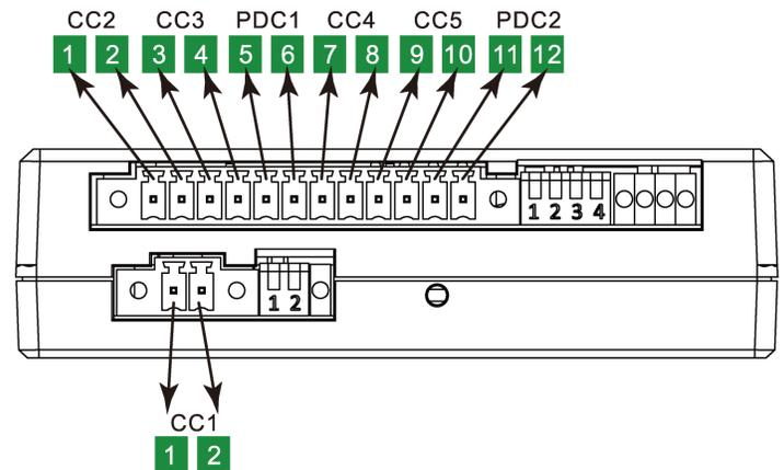
2. View the channel name above each pair of terminals on the label. A channel name comprises the terminal type and a channel number, such as CC1, PDC1, DC1, and the like.
