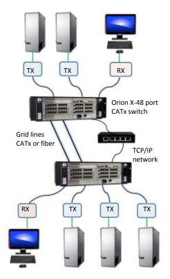
Structure of a matrix grid network
